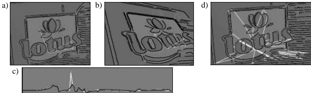
Figure 4 Projectively equivalent shapes (a), (b). Example of signatures (c) computed from these shapes. In (d) The “coverzone” of the signature in the original image is shown.
