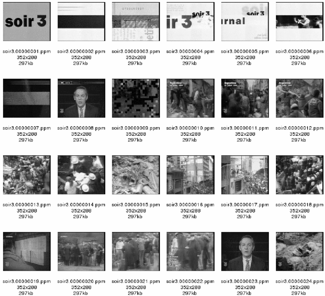
Fig. 5. Keyframes extracted from the 'soir3' sequence where the very long sequence with the commentator is as expected represented by a single keyframe
